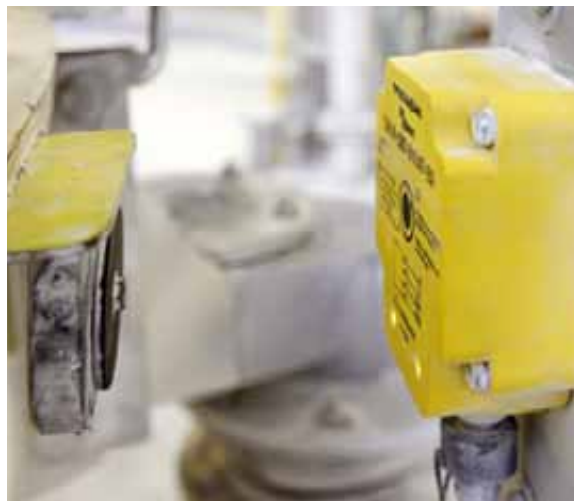
An Ex read/write head reads out the mesh width of the screen from the tag on the screen (left)
