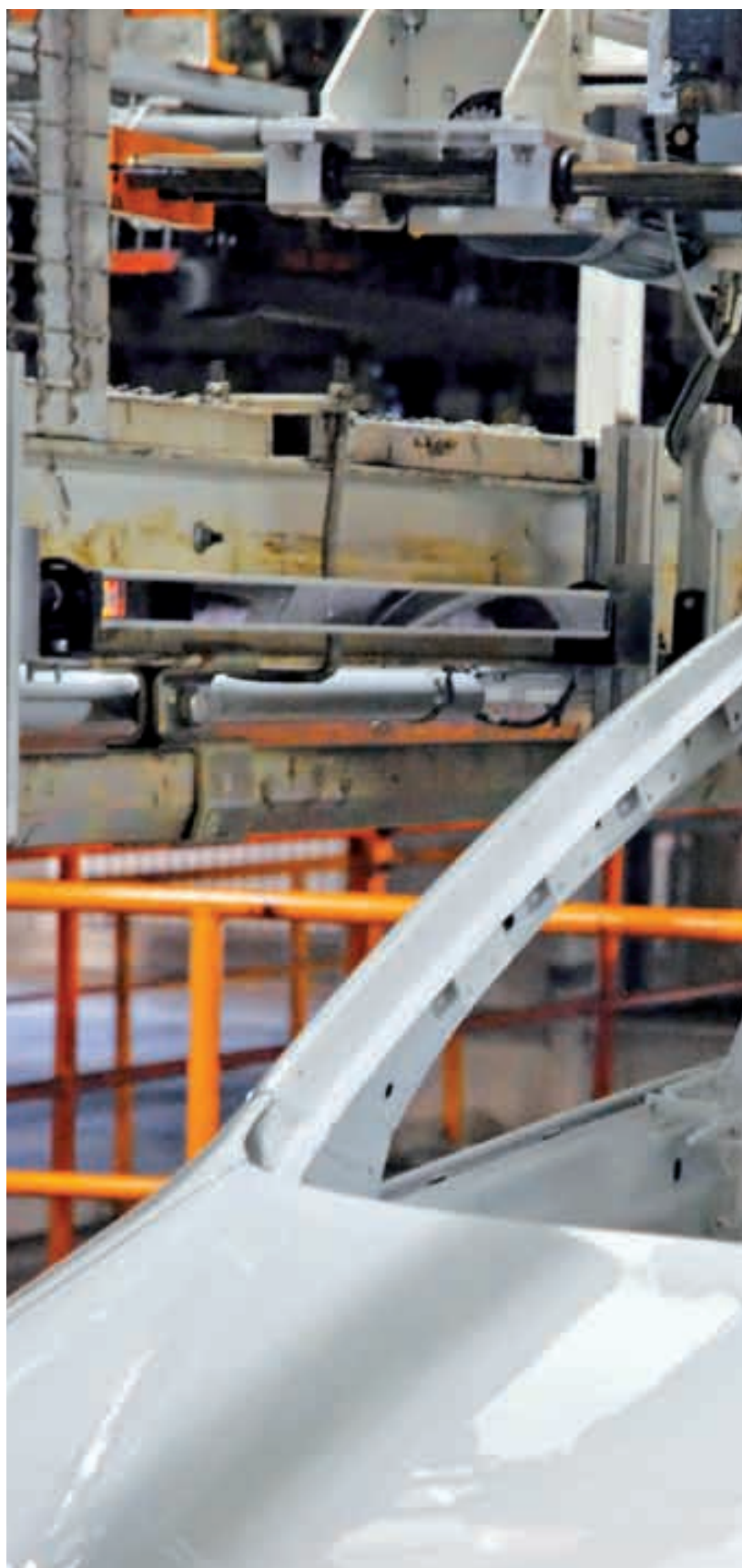
The EZ-Array measuring light curtains record the position of the car body and the grapple in real time
