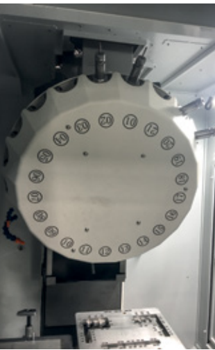
Tool turret with cutting tools
