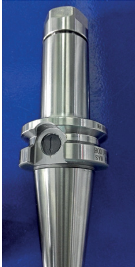
Cutting tool holder with embedded RFID tag
