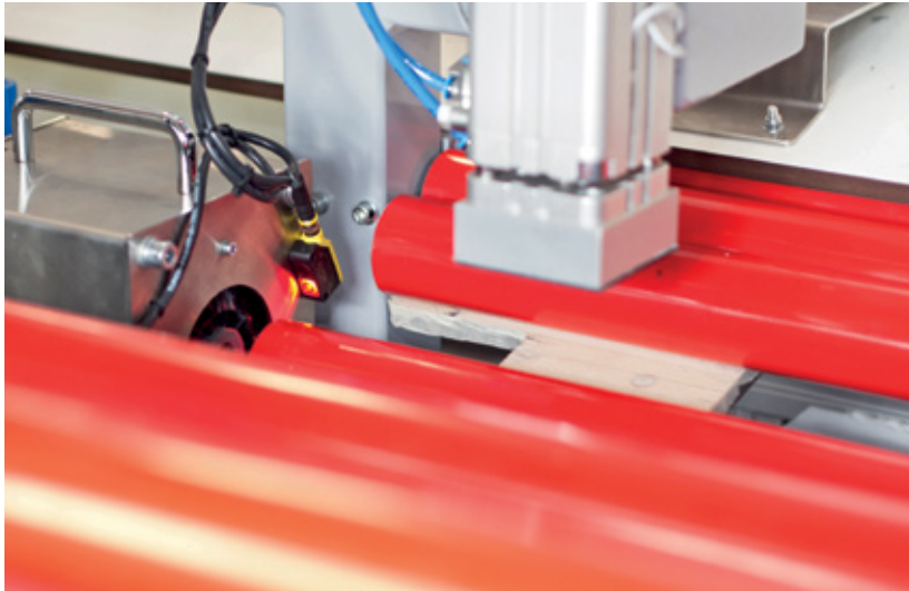
The Q20EQ7 infra-red sensor detects the join between two pipes
